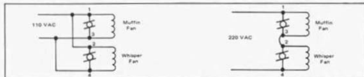
FIGURE 2-4. EXORciser Power Distribution Drawing
