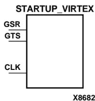
The STARTUP\_VIRTEX primitive is used for Global Set/Reset, global 3-state control, and the user configuration clock. The Global Set/Reset (GSR) input, when High, sets or resets all flip-flops, all latches, and every block RAM (RAMB4) output register in the device, depending on the initialization state (S or R) of the component.
