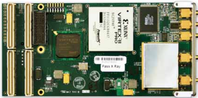
Figure 5 – UWB PMC module with dual 250 MSPS A/Ds
