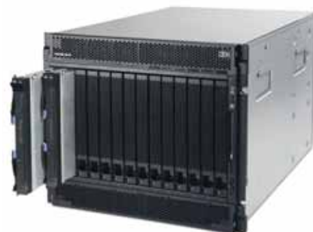
Figure 2 – IBM BladeCenter chassis with protruding Nallatech FPGA blade
