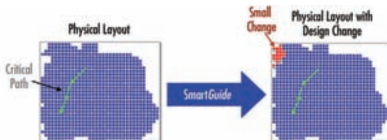
Figure 1 – SmartGuide can halve your place and route runtime. Small changes to RTL/constraints result in small changes to the physical layout, especially when the changes were not on the critical path.
