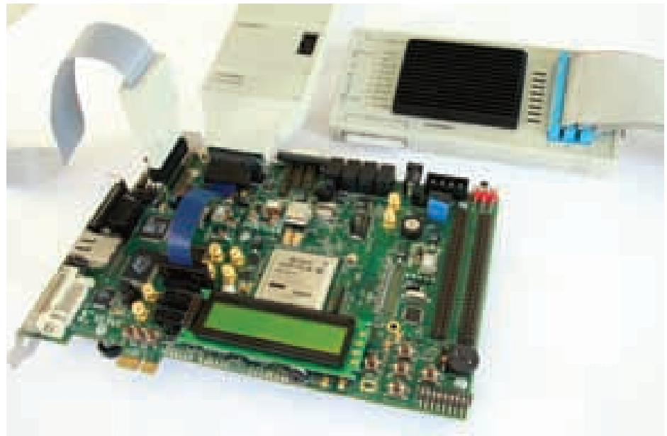
Figure 1 – Lauterbach TRACE32 debugging and trace cable connected to Xilinx ML507 board
