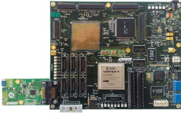
Figure 2 – A Virtex-4 FPGA sits at the heart of the WiLDSYS board.
