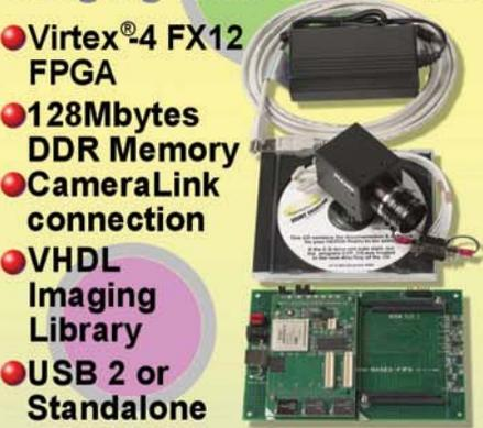
Programmable hardware with cables, device drivers, loading tools, examples and Power Supply. Systems can be used connected to a PC using USB, or can function standalone (without USB) using the initialisation PROMs.
