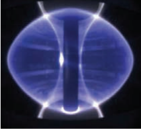
Figure 1 – The Mega Amp Spherical Tokamak (MAST) at CCFE is uniquely shaped, more similar to a cored apple than the traditional doughnut. The clear view inside the device shows the “bottled star” within.
