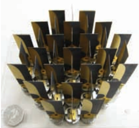
Figure 2 – The microwave-imaging phased antenna array utilizes novel PCB antennas.
