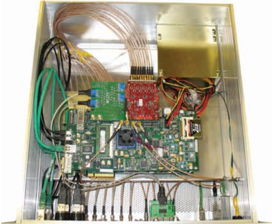
Figure 5 – The FPGA data acquisition box comprises Xilinx's ML605 evaluation board, 4DSP's FMC108 ADC board and our in-house FMC/PMOD header board. We wired the ADC SSMC connectors internally to front-panel SMA bulkheads to extend the life of the ADC analog connections.
