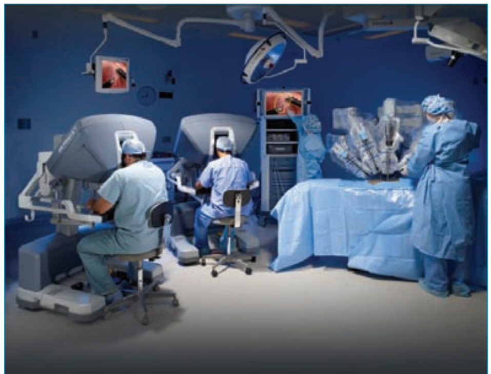
Figure 1 – The da Vinci System improves surgical outcomes and speeds patient recovery. In this picture, physicians sit at dual surgeon consoles, at the left and left middle. The vision system is pictured in the right middle, while the patient-side cart is at the right.
