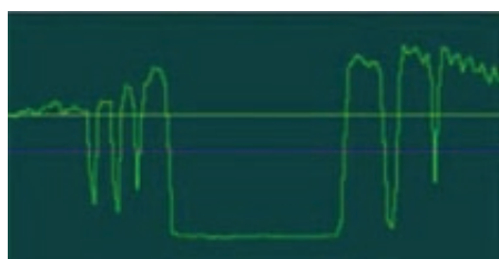
Figure 6 – Raw pixel line captured with a black line over a white background and some debris near it, before the thresholding and the salt-and-pepper filtering
