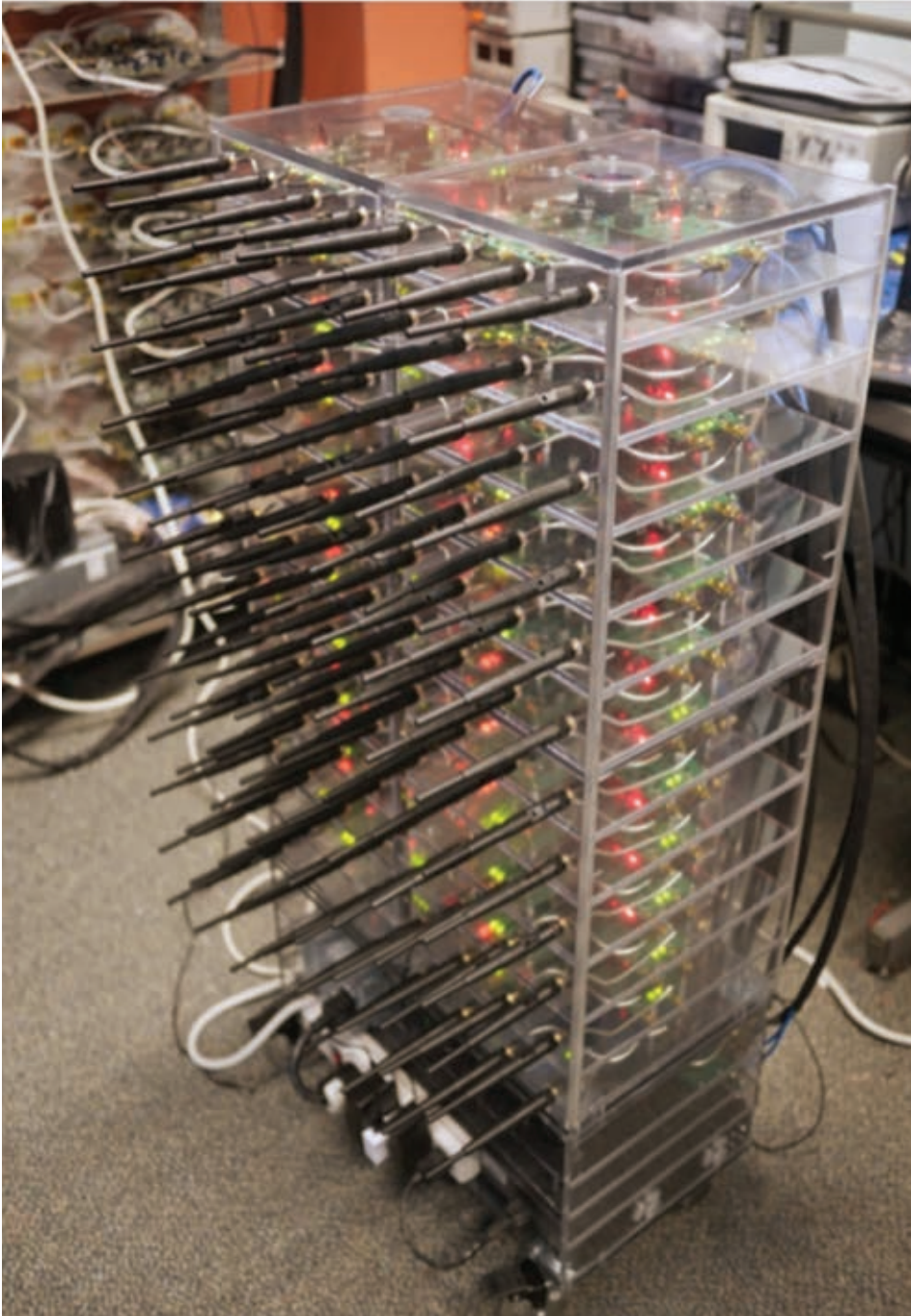
Figure 2 – The Rice University Argos v2 array combines 24 quad-radio WARP v3 nodes with shared clocking and Ethernet connectivity.
