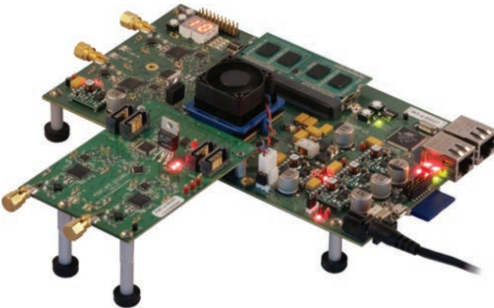
Figure 1 – The WARP v3 hardware with dual-radio FMC module provides a large FPGA, four RF interfaces, memory and two Ethernet connections.
