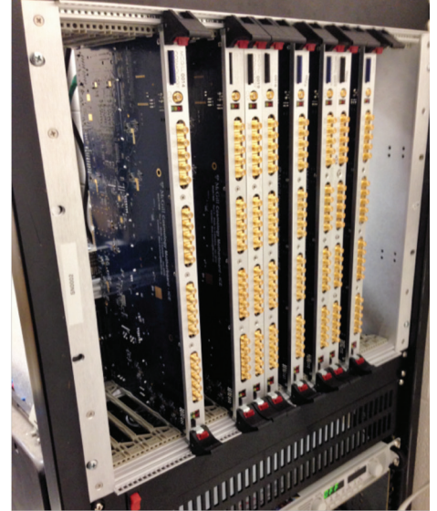
Figure 5 – This partially populated ICEBOX crate is part of the CHIME Pathfinder experiment.
