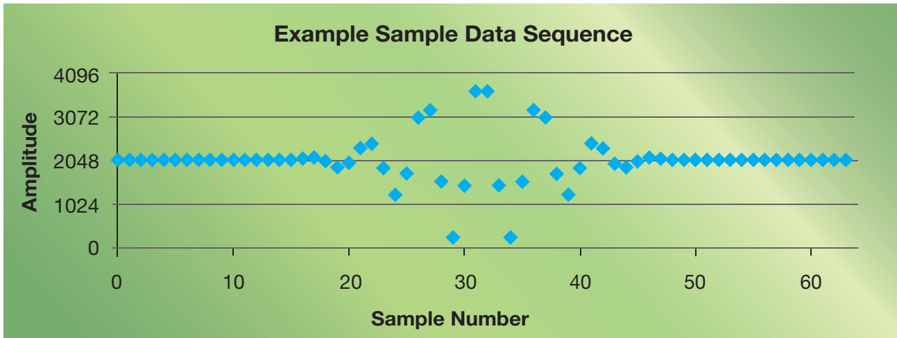
Figure 2 – Here is the example sample data sequence that results from sampling the example analog signal of Figure 1 at 80 MHz, or five times per period, using a 12-bit ADC driven to 97.7 percent of its full-scale input range.
