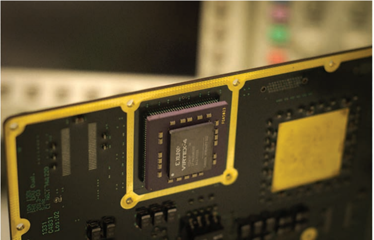
Figure 3 – Qualification board with soldered daisychain device
