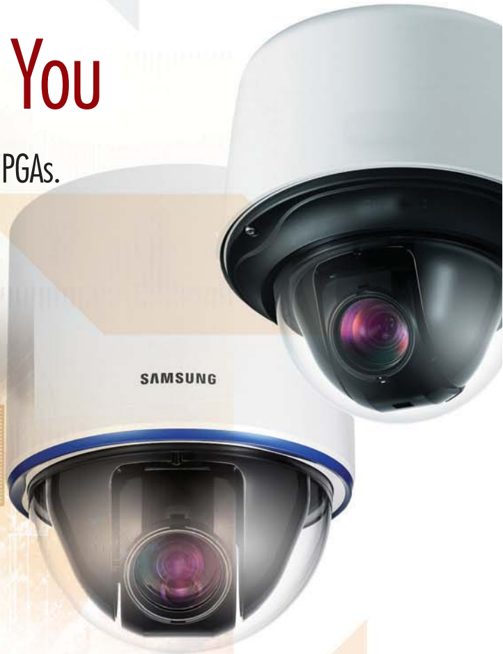
Samsung's dome camera uses a Spartan-3E with embedded MicroBlaze soft processor to calculate coordinates and interface with a digital video recorder.
