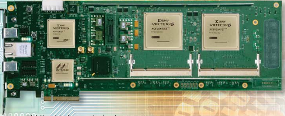
Dini Group's beefy prototyping boards pack 16 or more Virtex FPGAs.
