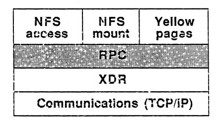
The XDR, RPC, and NFS protocols are all built on top of each other and on top of B-NET's TCP/IP communication facilities. Each of the NFS services accesses the underlying structure.
