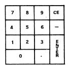
displayed and/or transmitted. The numeric pad includes a CE, Minus, and ENTER key. This group is a stand-alone numeric data entry key pad, not affected by the SHIFT, LOCK, or CONTROL keys.
