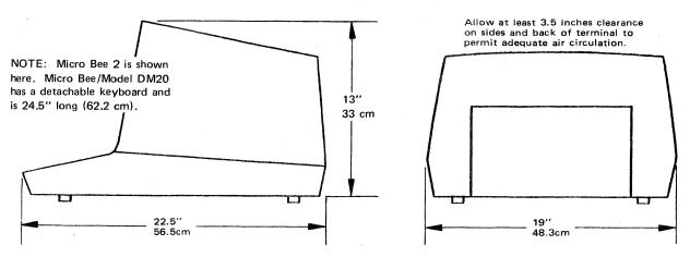
Figure 2-1 Mounting Requirements
