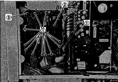
① Connector                      ② DC controller PCB
