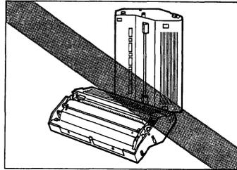
Figure 4-18 Bad examples of placing the cartridge
