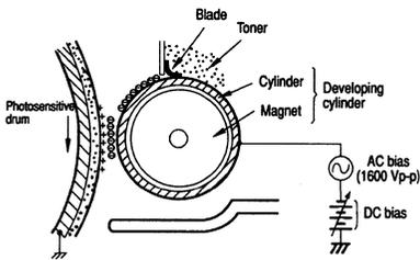
**Note:** The charges on the exposed area on the photosensitive drum are shown as positive in the above figure. Though they are actually negative charges, they are more positive than the developing cylinder so explanation of the developing stage is simplified by regarding them as positive.
