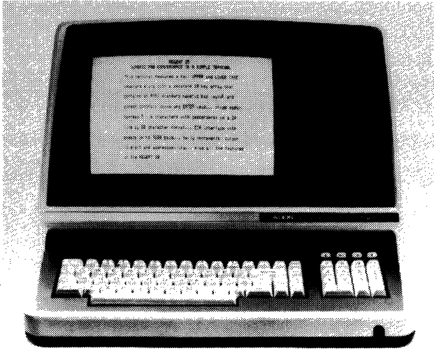
The Regent 25 has a display capacity of 1920 characters in a 24-line by 80-character format. The typewriter-style keyboard features a separate numeric and cursor control pad.
