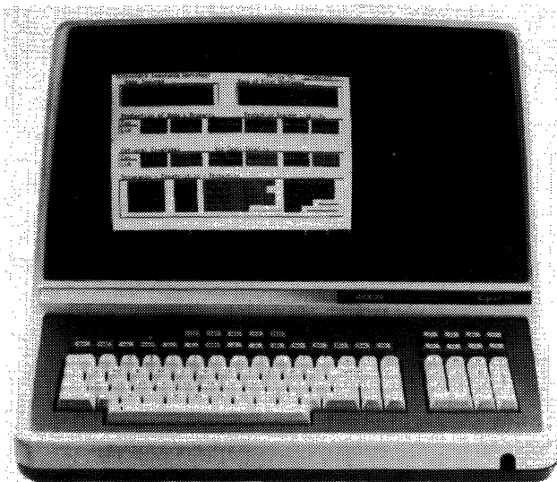
The Regent 60 is a smart buffered display terminal which can operate in conversational, message, or page modes.
