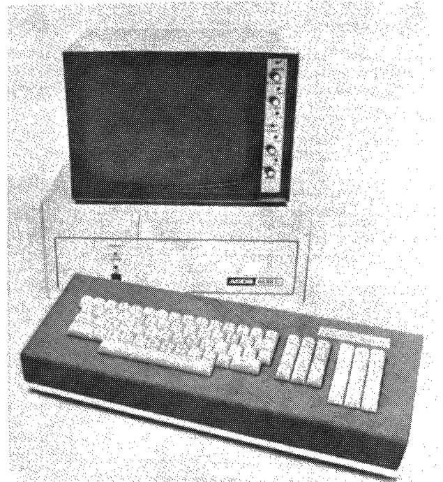
➤ This MRD Series 980 is designed for a standard 19-inch equipment rack and has three components: a 12-inch 1920-character monitor, a Teletypewriter-style keyboard with a numeric cluster and control pad, and the controller.
