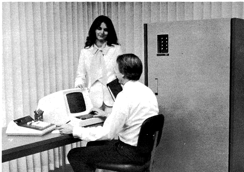
Memorex 1380 Communications Processor with attached Control Console and Systems Console (CRT). The Control Console is attached directly to the memory bus and is basically used by field engineers and programmers. The Systems Console is attached to a 1380 communications line port and is primarily for operator use.
