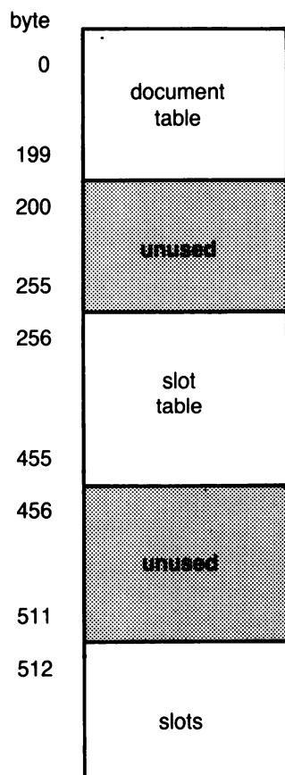
**Example** Suppose the WPS user creates document number 47. Checking through the slot table, WPS finds that the first free slot is slot number 22. In the document table, WPS changes byte 47 from 0 to 22. In the slot table, WPS changes byte 22 from 0 to 47. Then WPS copies the first 32 bytes of the new document's header into the 22nd slot.
