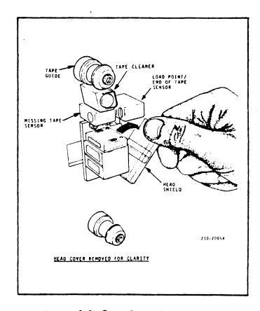
Figure 4-1. Opening of Head Shield
