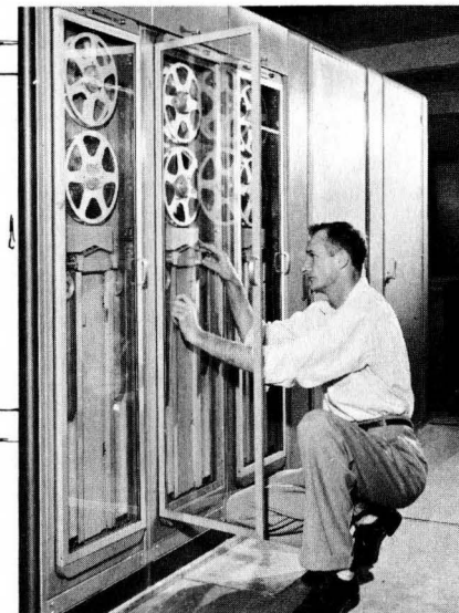
Keys to ERMA's operation are these units. Artist's conception at left shows typical input station with some of ERMA's panel boards in background. Picture at left shows one of the magnetic drums which temporarily stores activity information. In center is one of hundreds of electronic packages which do ERMA's "thinking." Magnetic tapes at right provide permanent storage of account information
