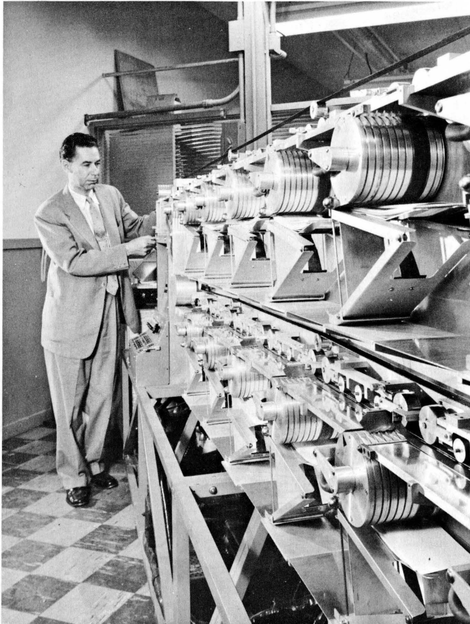
Dr. Kenneth R. Eldredge, manager of the Control Systems Laboratory, stands by the input station of the automatic check sorter, which "reads" account identification codes magnetically and sorts checks at a rate of 10 per second. The sorter rejects checks which have no magnetic code identification—as in the case of counter checks—and these are then handled manually. The check sorter automatically verifies its own "reading" accuracy by means of built-in checking features of the magnetic code itself and within the machine. The sorter misreads less than one in 10,000 checks and rejects less than one percent due to mutilation of codes or paper
