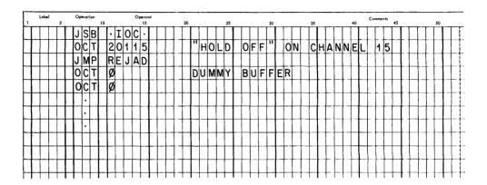
Abinary input operation must have a 2-word buffer. Thirty-two bits (8 BCD characters) are read directly into the 2-word buffer.
