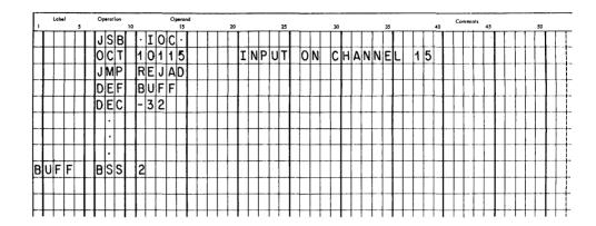
An ASCII input operation must have an 8 word buffer. 8 BCD characters are converted into 16 ASCII characters in the following format:
