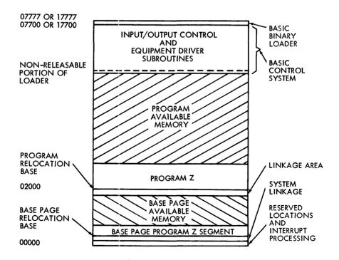
Options selected during PCS processing can define the equipment driver subroutines and other system routines as relocatable programs. If selected, these routines would be allocated to the available memory areas, and the length of the absolute segment of BCS reduced accordingly.
