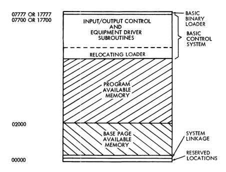
Assuming Program Z is to be loaded and executed – after loading, the memory might be allocated as follows:
