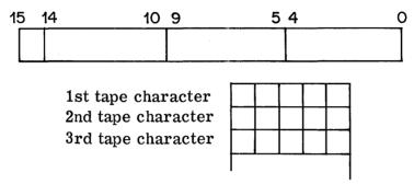
For output operations, the minimum buffer length is 3 computer words.
