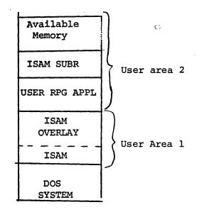
User application is initiated from console or batch. The user RPG application requests ISAM via a call to the ISAM subroutine which in turn translates into a DOS system call.
