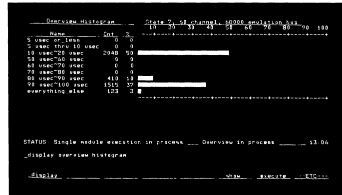
Figure 14. Interval overview allows rapid detection of spurious execution times, and is a powerful software characterization technique.
