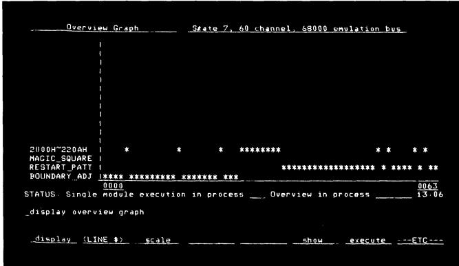
Figure 11. The sequential order of overview events is pictorially represented in the graph mode.
