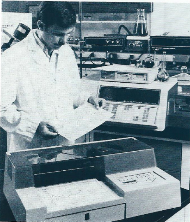
The new HP 7550A Graphics Plotter can be slaved to equipment such as this UV/visible spectrophotometer to produce hardcopy output of measurements. Featuring REPLOT firmware and automatic cut-sheet media feed, the HP 7550A is designed for unattended, automatic plotter applications.
