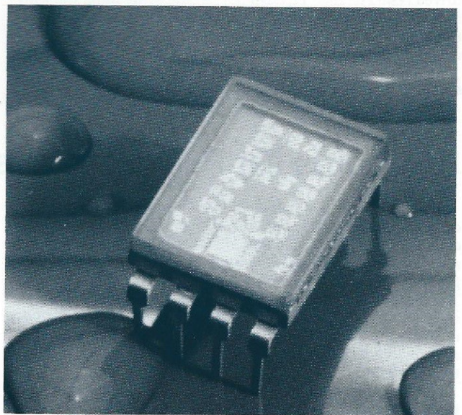
This new hermetic display, available in high-efficiency red and yellow, conforms to requirements for U.S. military applications.
