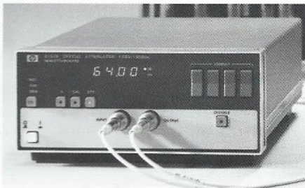
The HP 8157A Optical Attenuator provides more than 36-dB return loss.
