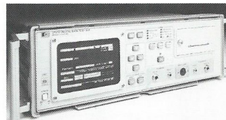
The new HP 3787B offers a single-unit solution to T1 and DDS/dataport test needs in the areas of production, installation, commissioning, and maintenance.
