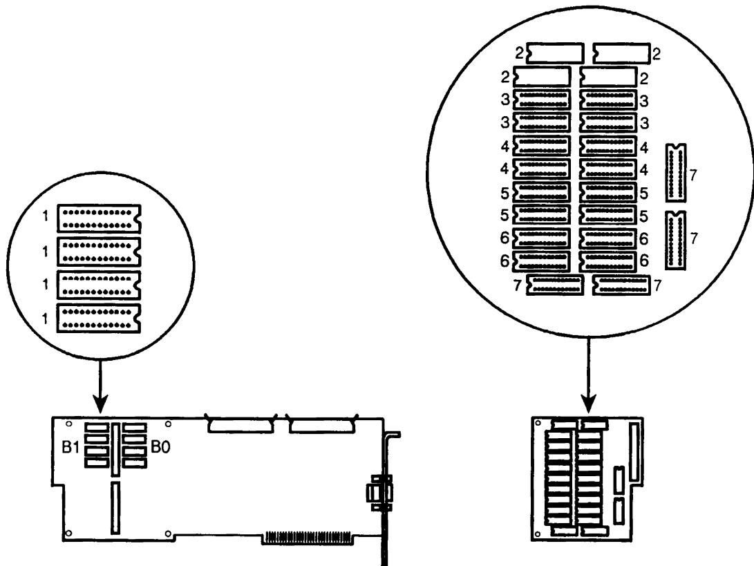
The HP 82303 RAM Expansion Kit provides one 512 KB block (four ICs) of RAM. You can install up to five of these RAM kits on the HP 82305 RAM Expansion Board. (Refer to the preceding figure for the location of each RAM block.)
