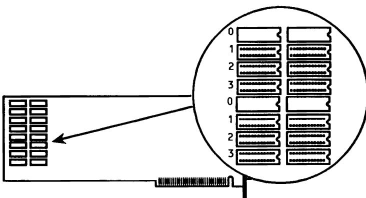
The HP 82303 RAM Expansion Kit provides one 512 KB block (four ICs) of RAM. You can install up to three of these kits on the graphics controller. The procedure for installing RAM ICs on the graphics controller is essentially the same as for the HP 82321 Language Processor, except that all of the ICs are installed on the graphics controller itself. No RAM expansion board is needed. Also, there is no RAM configuration switch on the graphics controller (it configures itself).
