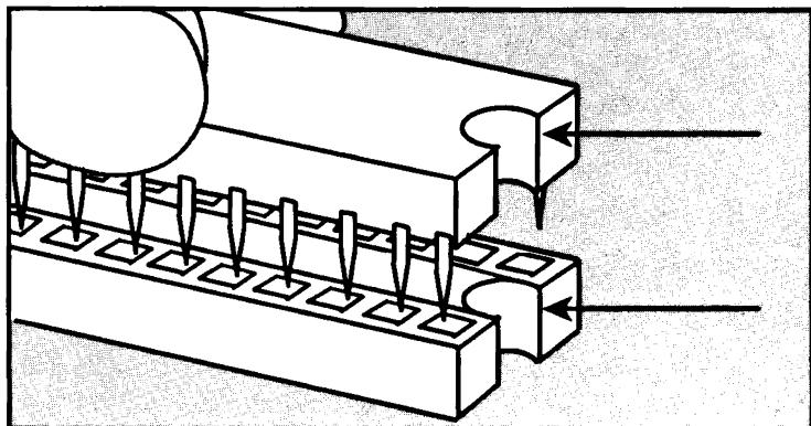
6. Align all of the pins on the IC with the holes in the socket. When properly aligned, press down on the IC until it is fully inserted. If any pins are not properly inserted, remove the IC and repeat this step.
