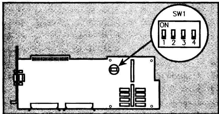
Determine which blocks of RAM are present (including the RAM on the RAM expansion board). Set SW1 as shown in the following table.
