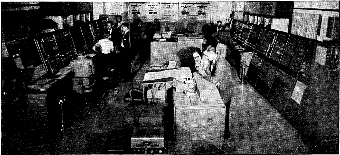
Figure 16. Control console. Separate control consoles (including standard IBM punched-card equipment) and magnetic-tape units are provided for each of the duplexed computers.
