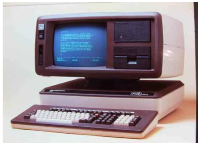
Fig. 3 A DRS20 model 25 Function Processor system, showing the single 5¼” diskette drive and the 5¼” hard drive housed in the display head.
