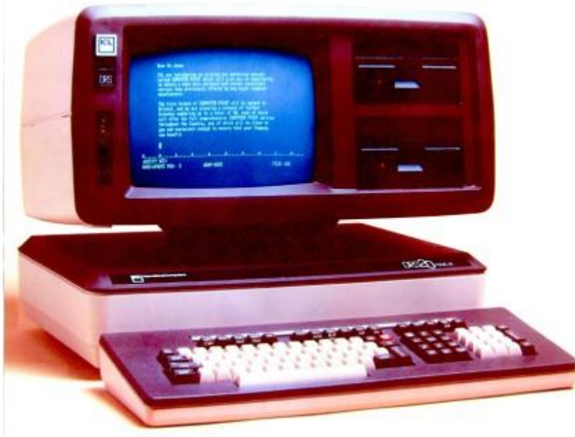
Fig. 2 A DRS20 model 20 Function Processor system of 1982 : The photo shows the distinctive keyboard design and the double 5¼” mini-diskette drive within the display cabinet.
