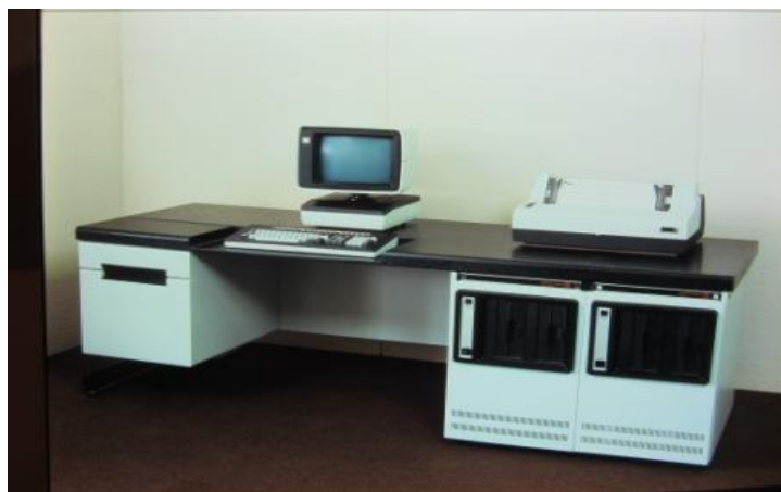
Fig. 1 A DRS20 model 40 Function Processor system, showing the two 8" floppy disk systems in one cabinet, also the extension cabinet housing two further 8" disk systems (note: this is the maximum disk system capacity for the original model 40).
