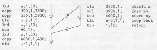
One feature which is poor about this program is that so much unnecessary data movement is required. For example, about 0.275 seconds data movement is required before entering the subroutine and about 0.175 seconds data movement is required after exiting from the subroutine---and only 50 points were moved. Another poor feature is that a maximum of 100 points can be multiplied together since only that much temporary working space has been allocated at the end of the memory.
