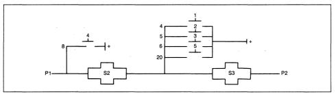
Using the chart provided in Appendix B, locate the diagram corresponding to the final position of S2, S3 and S4. This illustrates the pin or pins requiring pull-up jumpers when building a custom cable.
