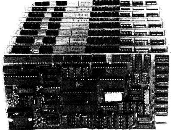
MDZ Computer systems are expandable to as many as sixteen users. To add a user simply plug in a slave processor board, add cables and a terminal.
