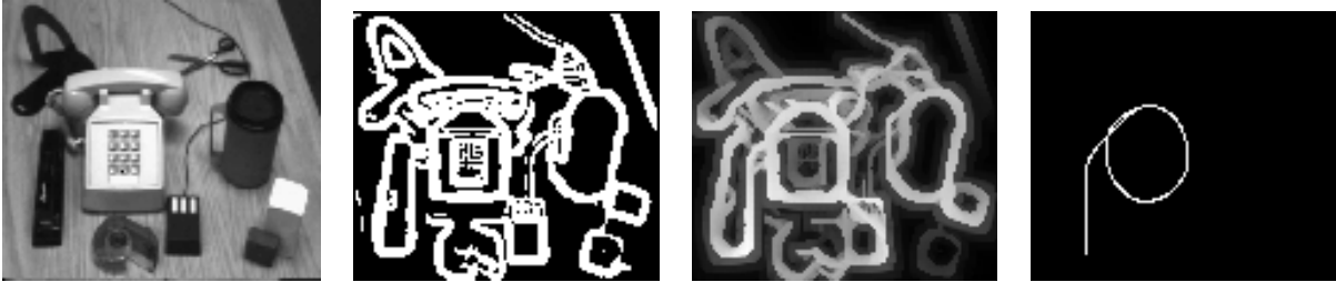
Figure 11: Shashua and Ullman’s saliency map for a cluttered scene. From left to right, the first picture is the scene image and the second is an edge image obtained from the scene image by thresholding the gradient magnitude. The edge image was the input to the network. The third picture displays Shashua and Ullman’s saliency map, and the fourth shows the curve (51 elements) emanating from the most salient element, for which \Phi = 210.1 .
