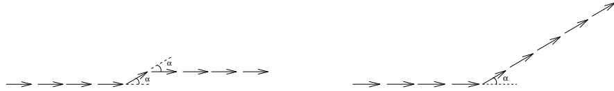
Figure 8: Discretization effect on a straight line. Left figure: the discretization of a straight line. Right figure: a corner. The saliency value obtained for a perfectly horizontal line of length 20 is 20.00, the saliency value for a straight line of the same length is 18.41, and the saliency value of a corner is 19.10.
