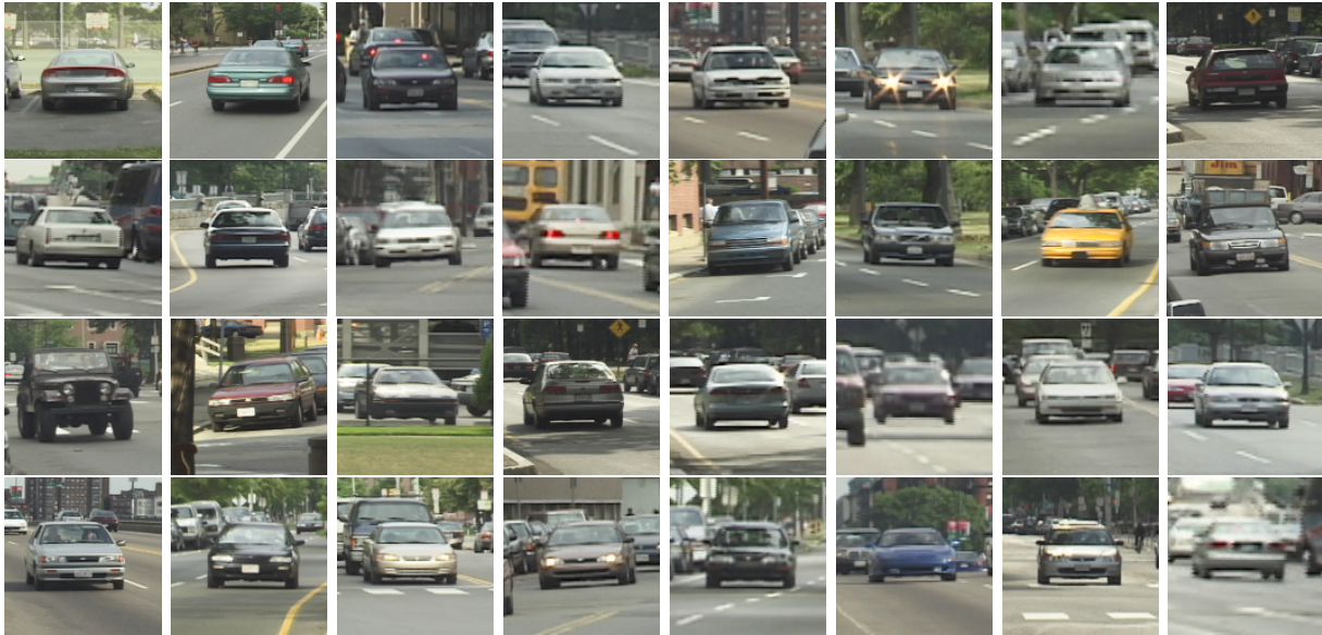
Figure 1: Examples from the database of cars used for training. The images are color of size 128 \times 128 pixels, normalized so that the front or rear bumper is 64 pixels wide.
