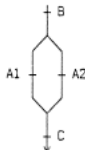
Fig. 6: Two identical pieces of code at A1 and A2 can be factored forward to position B, or backward to position C, as long as the new position is consistent with data flow constraints.
