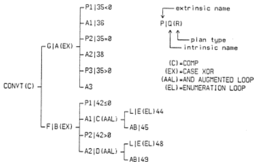
Fig. 29: Schematic of the grand plan for CONV T. This is a shorthand notation for a diagram of the grand plan similar to the diagrams for the plan types in section III.3. This figure shows how the plans are imbedded. The diagrams in section III.3 show what the diagram corresponding to each node of the schematic looks like.
