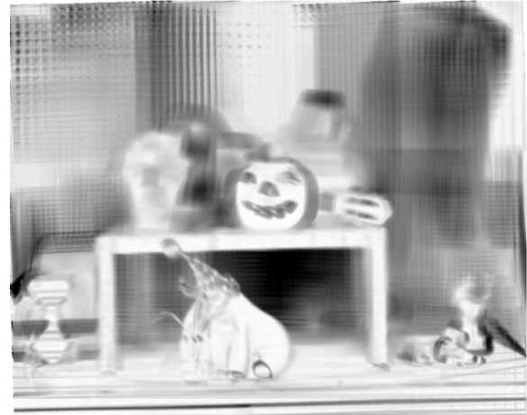
Figure 15: Here is a visualization of the scores used on the front focal plane for the picture in Figures 11 and 20. The closer to white, the better the score \sigma , which means objects are likely to be located near that plane.
