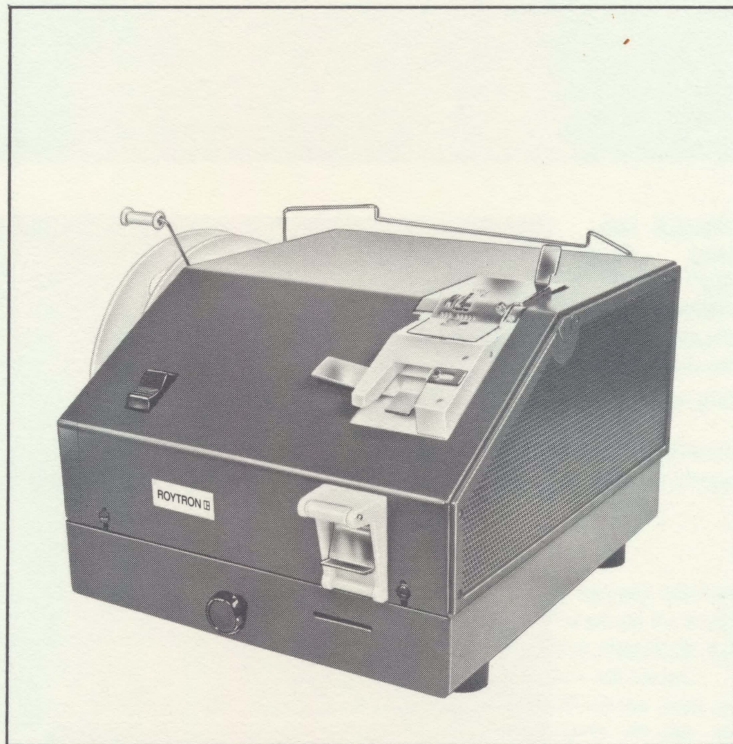
Roytron Series 500 and 700 Integrated Read Stations can operate as a complete tape read facility. In this configuration, an 8 1 / 2 " reel of punched tape is placed into the drawer mounted at the base of the unit. The tape feeds through the read head and a tape guide (located at the rear) to a side mounted take up reel. Take up reels in either 7 1 / 2 " or 8" diameters are available. Overall dimensions are: 13 1 / 2 " wide x 15" deep x 9 1 / 2 " high. Weight is approximately 23 1 / 2 lbs.
