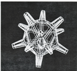
This type of drawing is a "wire frame" of a ship mine.
