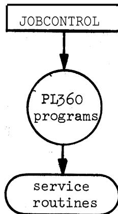
The jobcontrol program and the service routines are executed in the supervisor mode and are storage protected. Together they occupy the first 8000 bytes of core memory.
