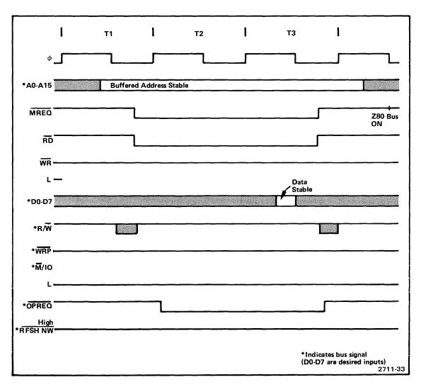
Fig. 9-4. Assembler Processor Memory Read Timing.
