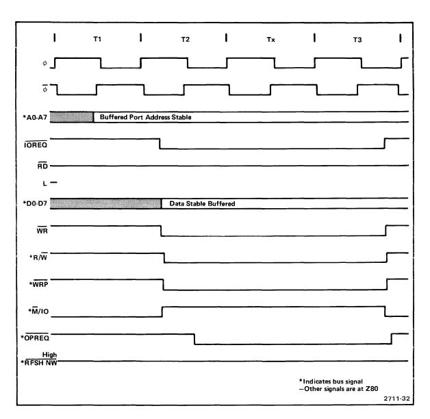
Fig. 9-3. Assembler Processor I/O Write Timing.
