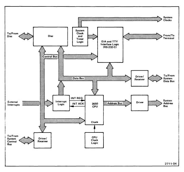
Fig. 1-3. 8001/8002A  $\mu$ Processor Lab System Processor Block Diagram.
