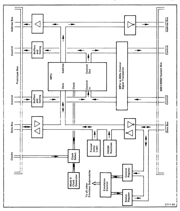
Fig. 1-4. 8001/8002A  $\mu$ Processor Lab Emulator Processor Block Diagram.
