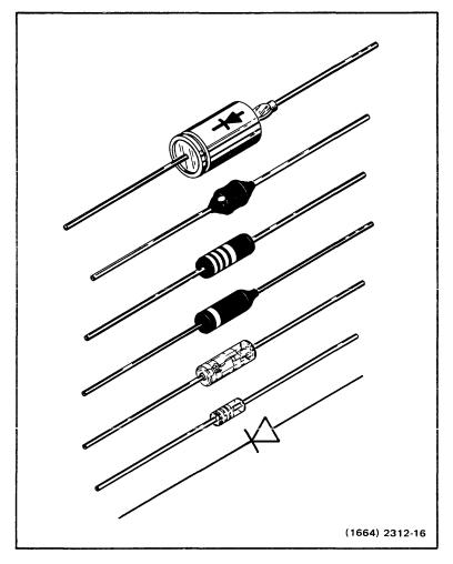
Fig. 11-2. Diode Polarity Marking.
