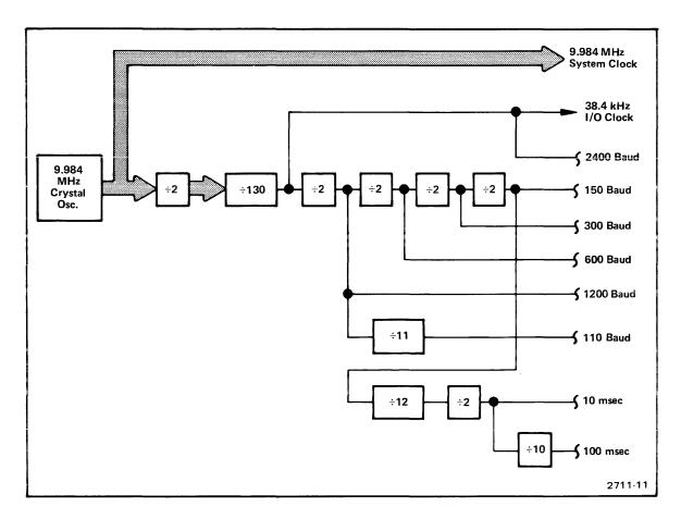
Fig. 3-2. Baud Rate Clock Divider.
