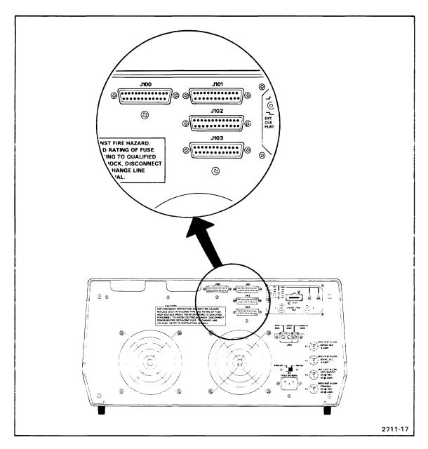
Fig. 5-3. 8001/8002A μProcessor Lab RS-232-C I/O Ports.
