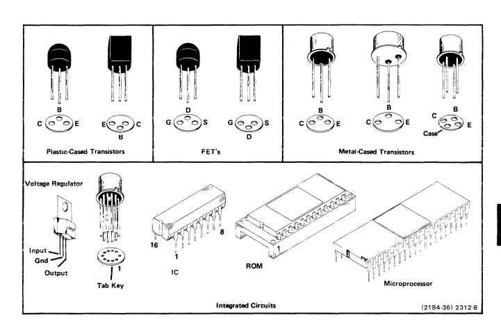
Fig. 11-3. Pin Configuration for Semiconductor Components.
