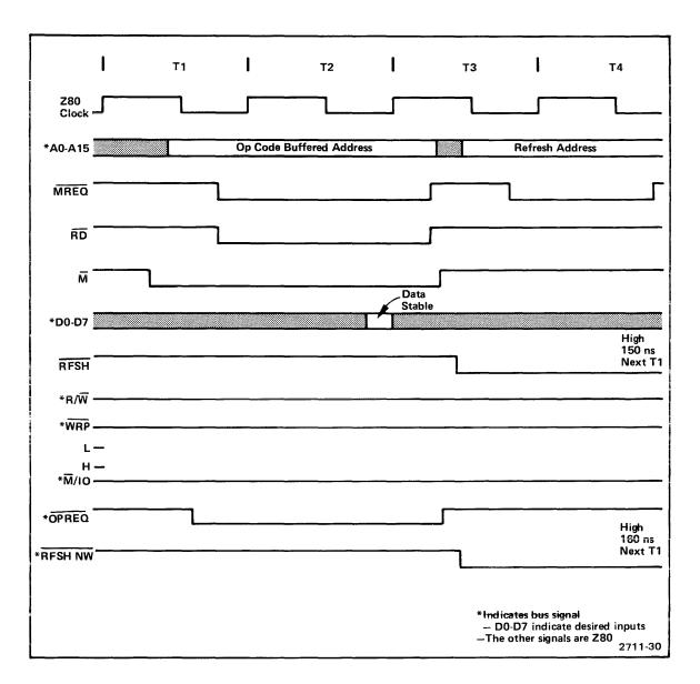
Fig. 9-1. Assembler Processor Operation Code Read Timing.
