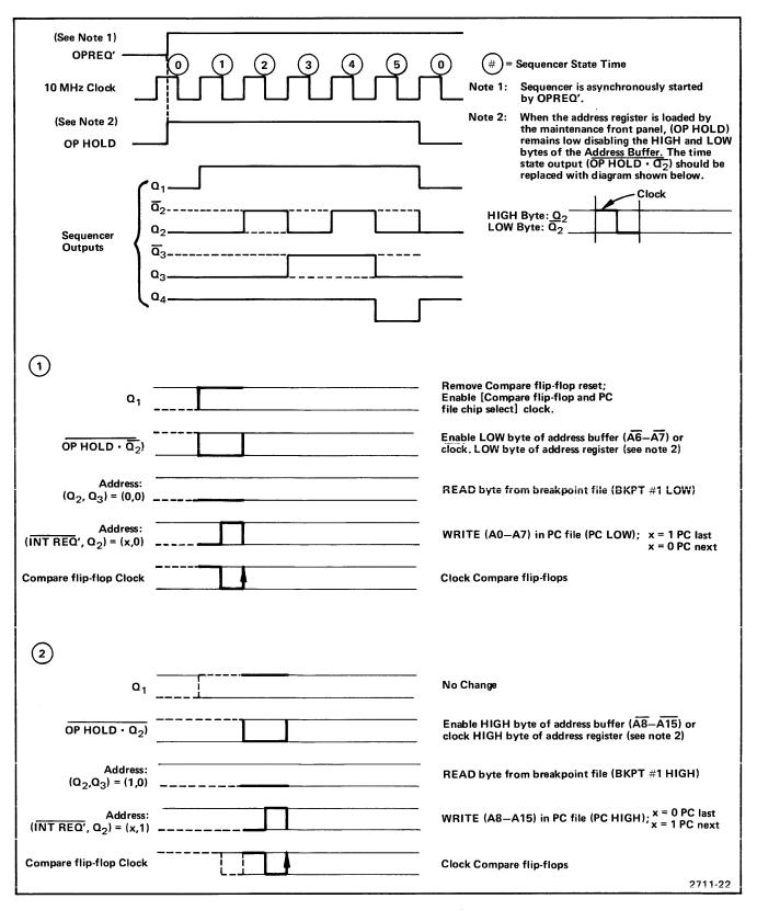
Fig. 6-3A. Sequencer State Timing Diagram.
