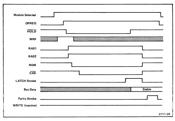
Fig. 8-6. High-Speed Memory Read Cycle.
