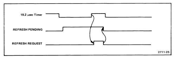
Fig. 8-2. Asynchronous Refresh Timing for High-Speed Memory.
