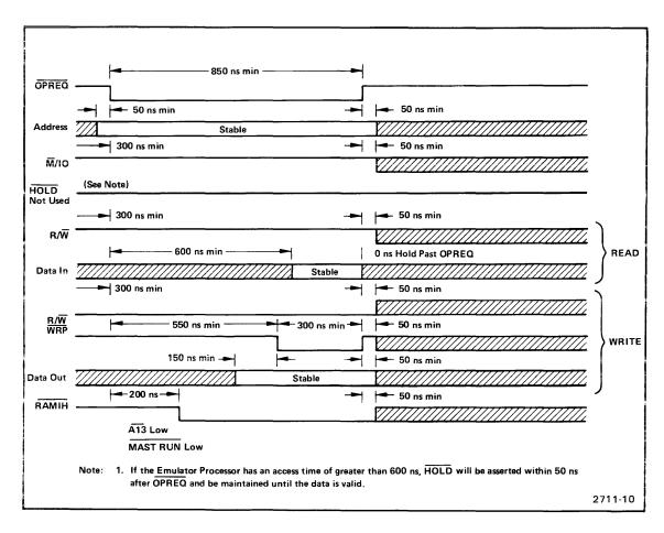
Fig. 3-1. System Processor M/IO Read and Write Timing Diagram.
