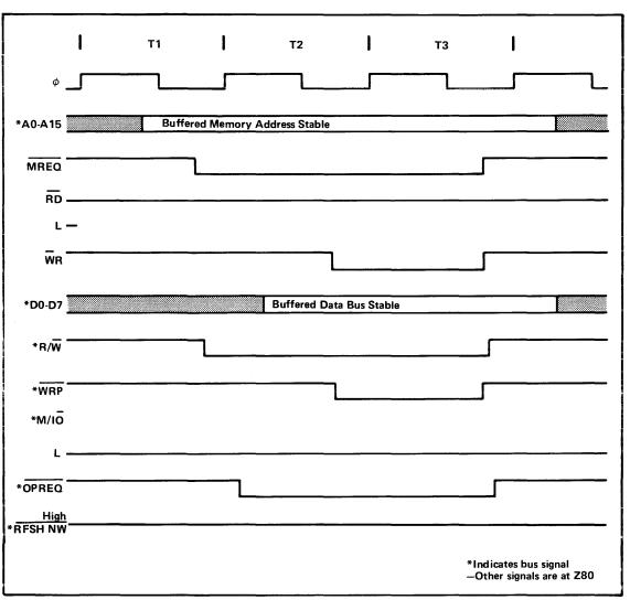
Fig. 9-5. Assembler Processor Memory Write Timing.
