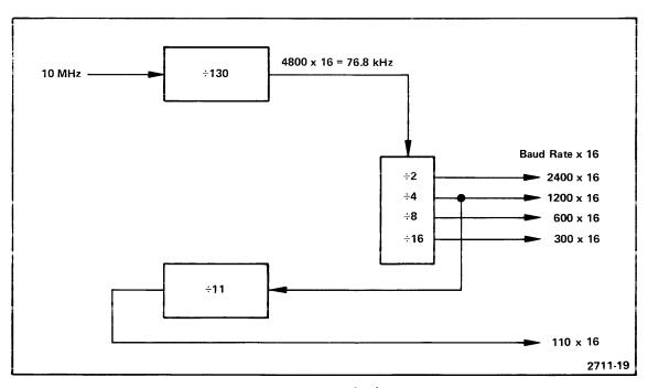
Fig. 5-1. Baud Rate Logic.
