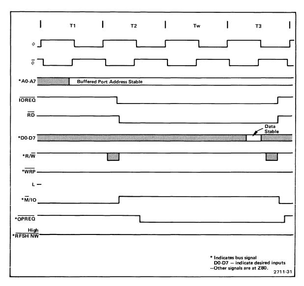
Fig. 9-2. Assembler Processor I/O Read Timing.
