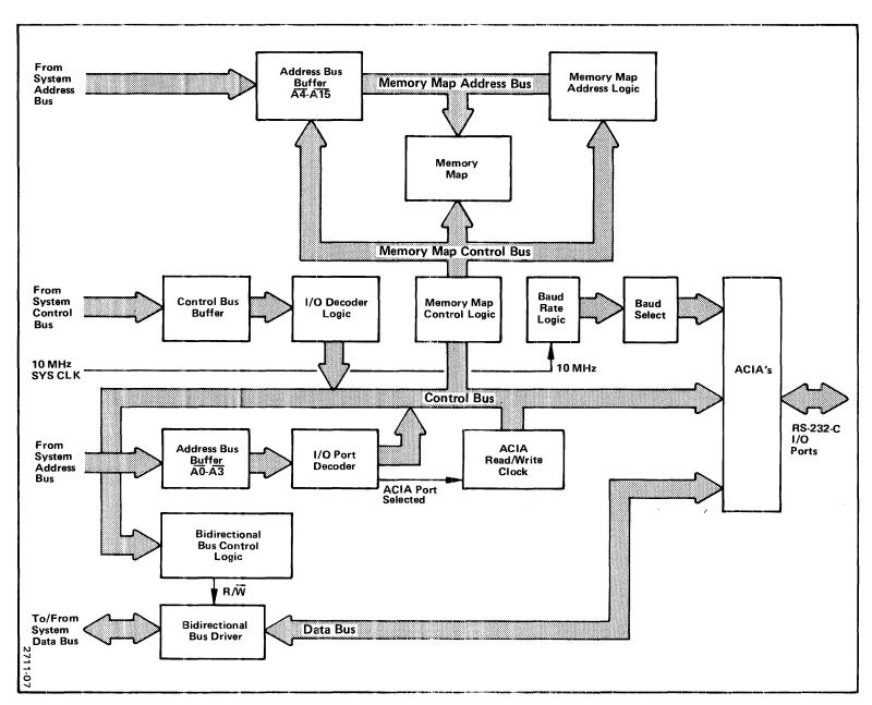
Fig. 1-6. 8001/8002A μProcessor Lab System Communications Module Block Diagram.
