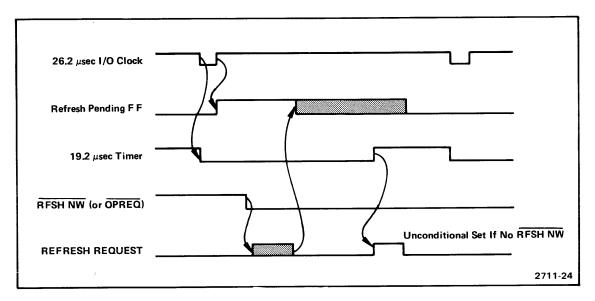
Fig. 8-1. Refresh Timing for High-Speed Memory.
