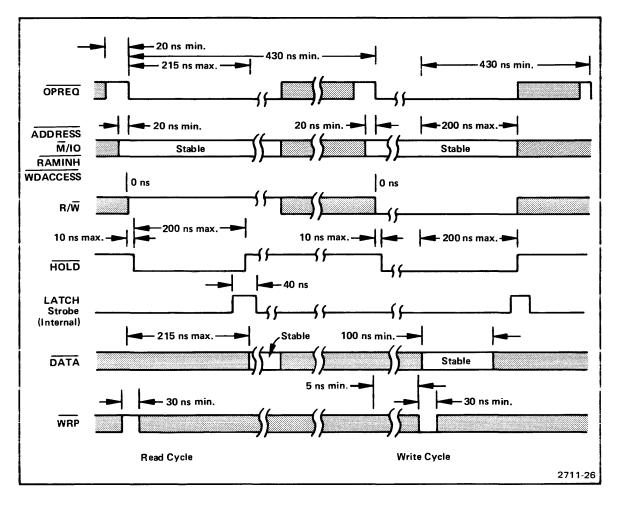
Fig. 8-3. High-Speed Memory Timing.
