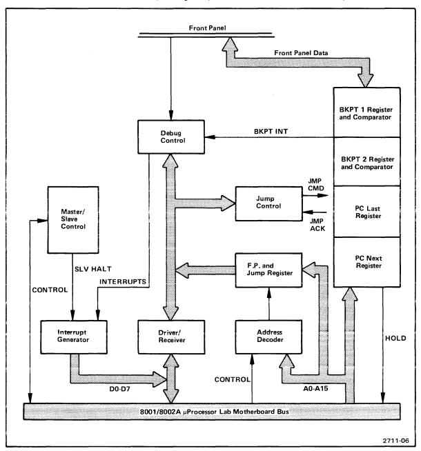
Fig. 1-5.  $8001/8002 \text{A} \, \mu \text{Processor Lab Debug and Front Panel I/O Module Block Diagram}.$
