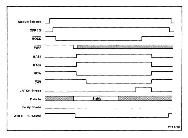
Fig. 8-5. High-Speed Memory Write Cycle.
