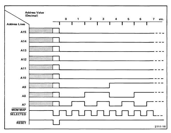
Fig. 5-5. Memory Map Address Logic Timing.
