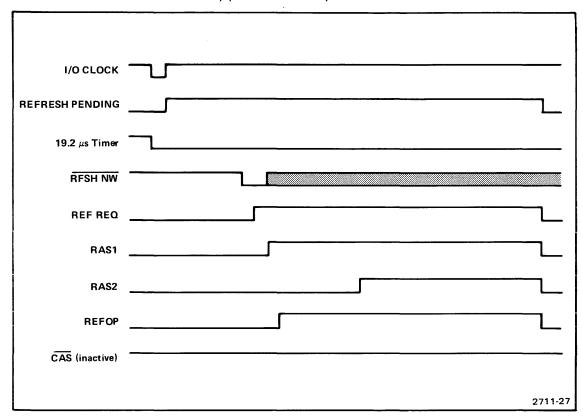
Fig. 8-4. High-Speed Memory Refresh Operation.
