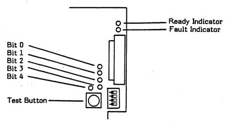
To read Status Codes, set Off-Line mode and press the Test Button. The last Status Code stored will be displayed. Up to 16 Status Codes may be stored.
