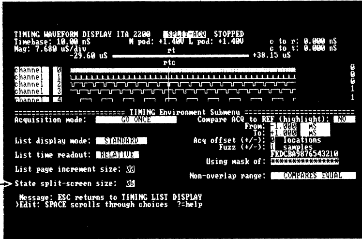
■ Figure 6-6. Selecting the size of the split-screen display in the timing analyzer's Environment Submenu.
