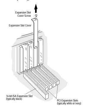
**Step 3:** Insert the host adapter in the slot; press down firmly so that the bus contacts are securely seated in the slot. Secure it with the screw you removed in Step 2.
