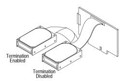
**Step 5:** Install and mount each internal SCSI device in an available drive bay inside your computer. (Refer to your computer and device documentation for instructions.)
