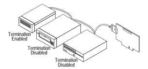
**Step 11:** Plug one end of the external SCSI cable into the host adapter's external SCSI connector and plug the other end of the cable into either one of the SCSI connectors on the external SCSI device. (If you are installing only one external device, attach a terminating plug to the device)
