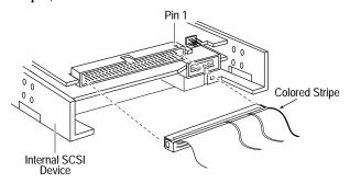
**Step 8:** Plug the remaining connectors on the cable into any remaining internal devices (these devices must not be terminated; see Step 4).
