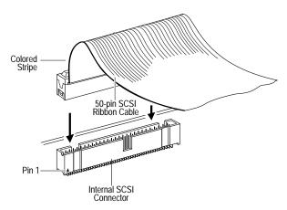
**Step 7:** Plug the other end of the cable into the last internal device (this device must be terminated; see Step 4).
