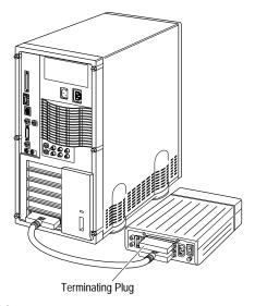
**Step 12:** Connect other external SCSI devices by daisy-chaining each device to the previous device until all external SCSI devices have been connected. (The device at the end of the chain must have a terminating plug installed.)
