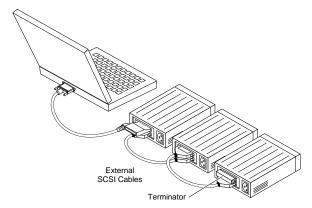
5 Make sure that each SCSI device has a unique SCSI ID from 0 to 6. For instructions on changing the ID for a device, see the device documentation.
