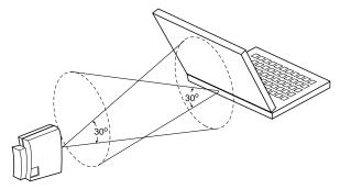
Be sure that both infrared devices are within this 30-degree cone. File transmission will fail if one of the devices is turned too far to the right or left or is much higher or lower than the other device.
