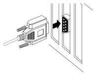
If your PC has a 25-pin connector, you must use a 9-pin-to-25-pin converter, as shown in the following diagram.
