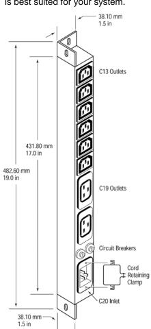
PDU E7671A may be used alone or in combination with another PDU from the modular PDU family.
