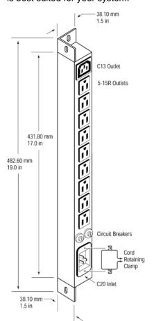
PDU E7675A may be used alone or in combination with another PDU from the modular PDU family. E7675A is designed for needing NEMA oulets on the PDU.
