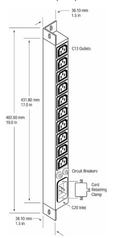
PDU E7676A may be used alone or What you get in the box in combination with another PDU from the modular PDU family. E7676A is designed for situations requiring only C13 outlets on the PDU.
