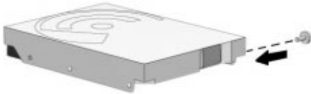
Figure 5-96. Installing the Flanged Screws into the Hard Drive
