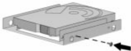
Figure 5-99. Inserting the High Hat Screw into the Bracket
