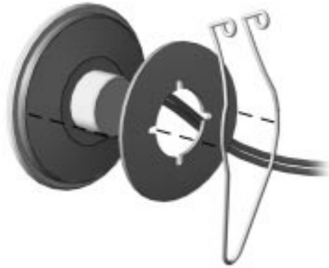
Figure 5-8. Installing the Cardboard Insulator and the Retaining Clip onto the Speaker
